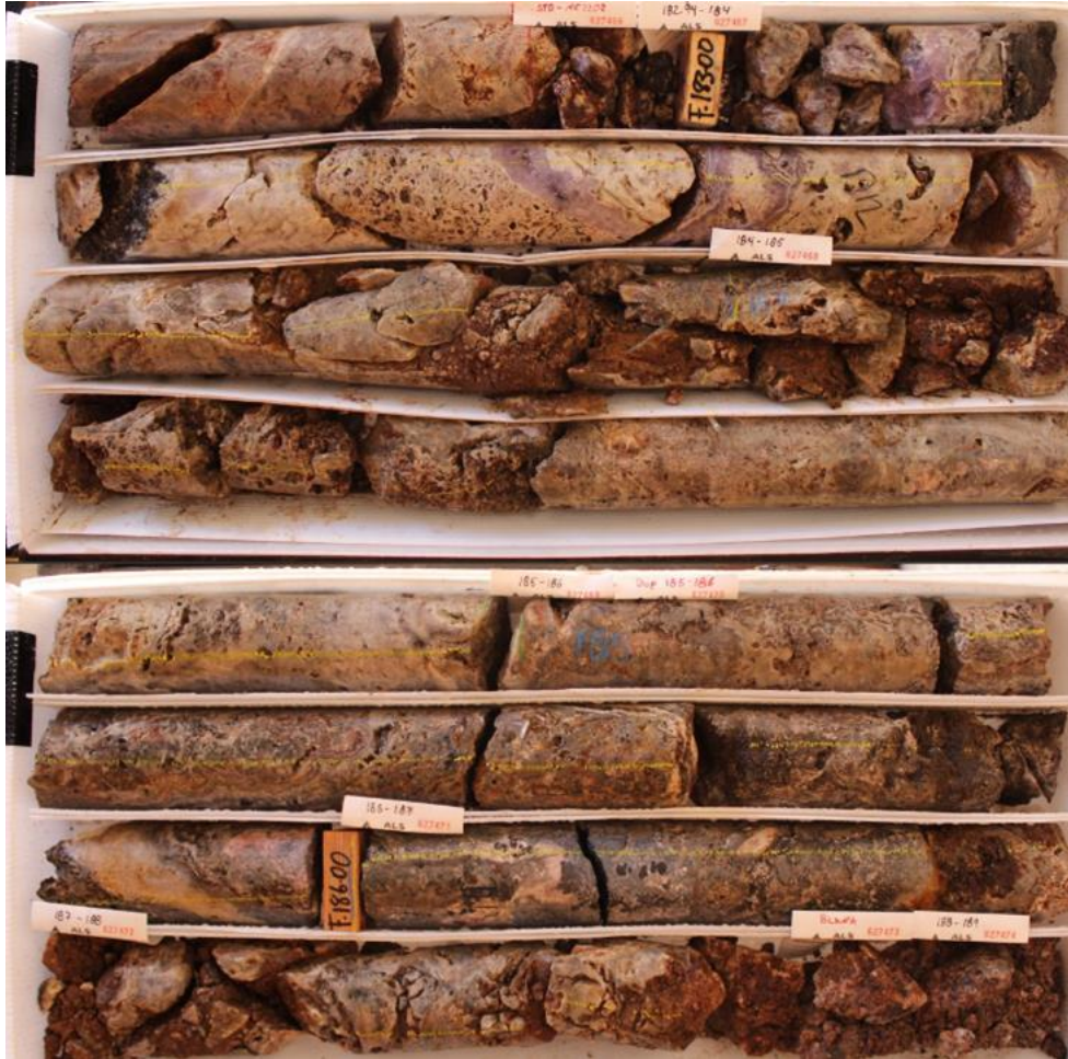
Photograph of initial portion of D Vein intercepted at roughly 183 m downhole in CDH-23-138*
